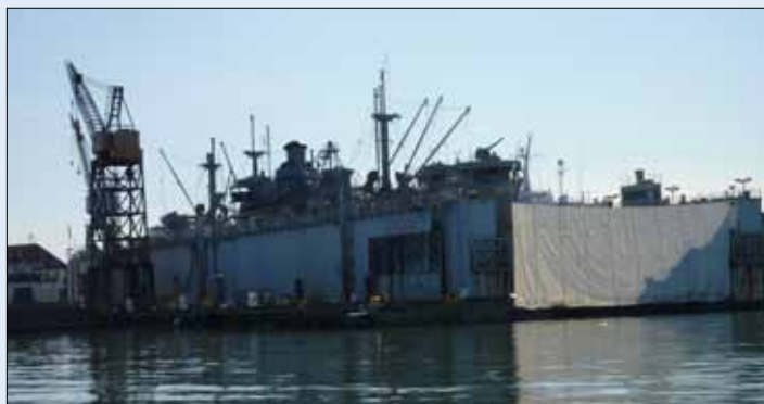
As a result of Baykeeper legal action, BAE Systems San Francisco Ship Repair, Inc. agreed to install new pollution controls. Above: When old paint is being sandblasted off ships at the BAE dry dock, newly-installed shrouding is designed to protect the Bay from toxic dust and particles.
